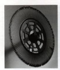
Apple printwheels are designed for high print quality and durability. Unlike manufacturers who place two characters on one spoke. Apple's printwheels have one spoke for each character. This eliminates shifting the carriage up and down, a major cause of wear and character misalignment. Apple has a complete line of plastic daisywheels, from Prestige Elite to Boldface in English, French, German, and many other languages, as well as offering proportional spacing.
