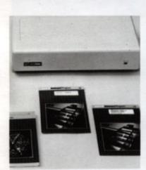
ProFile is the Personal Mass Storage System for Apple computers. ProFile is a complete storage system; it includes a 51/4-inch, Winchester technology hard disk housed in a compact, sealed environment; device driver software; and the ProFile interface card. The Personal Mass Storage System dramatically increases the Apple's maximum on-line storage capacity to 5 million bytes, allowing you to store safely in one location information that would fill 35 floppy disks.
