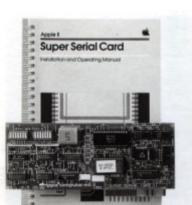
The Apple II Super Serial Card allows Apple II computer systems to exchange data with other computers, moderns, printers, terminals, and accessories, employing a bi-directional RS-232C interface in serial format (one bit at a time).
