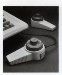
The Apple Hand Controllers //e are reliable, precision built game paddles which offer a new level of enjoyment to action oriented computer games. The dual diameter control knob allows control of the paddle from either diameter and the precision fire button with tactile feedback has been designed for long life and reliable operation. With the Apple Hand Controller //e you can just
