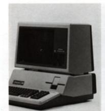
Apple's portable, 12-inch (30.5 cm) (diagonal), black and green monitor displays 80-character by 24-line text and high resolution graphics with precision and high readability. Designed for use with Apple III computer systems, it will also display 40 characters per line when used with Apple II Plus computers, or when the Apple III is operating in Apple II emulation mode.
