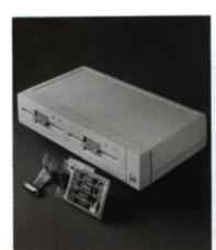
DuoDisk is a twin 143K, two-thirds height disk drive system designed for the Apple // family of computers. Its case is designed to the same width, colour and styling as the Apple // Amount of the transfer o
