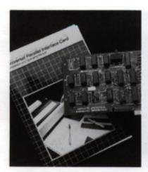
The Apple III Universal Parallel Interface (UPI) Card lets users attach a variety of parallel-mode printers — including most dot matrix models, plus some thermal and daisy wheel units — to Apple III computer systems. Included with the Card is a disk containing an operating system driver, which lets you custom configure the card to work with the printer you are using.
