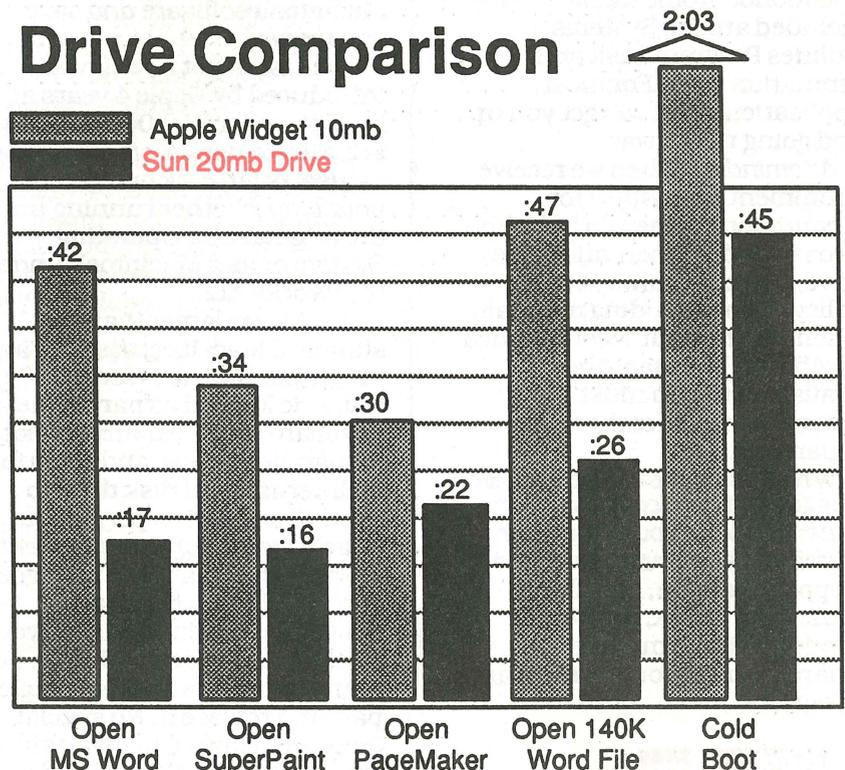
The new Sun 20 Hard Drive for the Lisa and Macintosh XL not only provides for larger storage capabilities than ever before but registers a significant increase in efficiency and speed.
