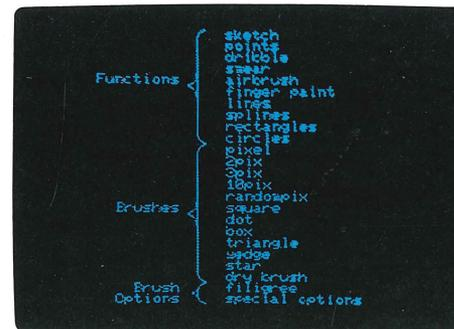
The Utopia Graphics Tablet System is highly interactive. Its menus, sub-menus, colors, and graphics options can be selected at the touch of your pen-controlled cursor. Simply press the pen down outside the tablet's grid whenever you want to enter a menu, and without menu overlays or keyboard commands, your menu will immediately appear. It lets you build a library of useful shapes to access quickly and use over and over again.
