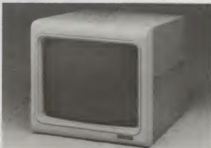
Quadscreen's 17-inch monochrome screen displays 10,240 characters — more than five times the screen capacity of IBM's PC monitor.
