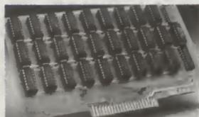
with the Professional Computer and each card is "burned in" and tested for quality control before being shipped.
