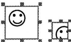
*After resizing a painting frame, the graphic is still positioned the same relative distance from the top-left of the frame.*
