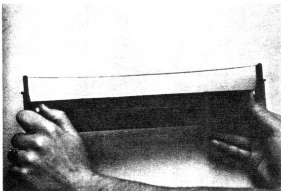
3. Take up any slack in the new ribbon by turning the knob on the cartridge counter-clockwise.
