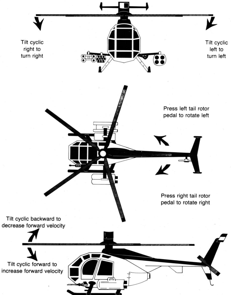
Figure 2. Helicopter Flight Control Surfaces
