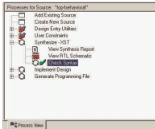
FIGURE 6-2: PROCESSES WINDOW SHOWING CHECK SYNTAX HAS COMPLETED SUCCESSFULLY
