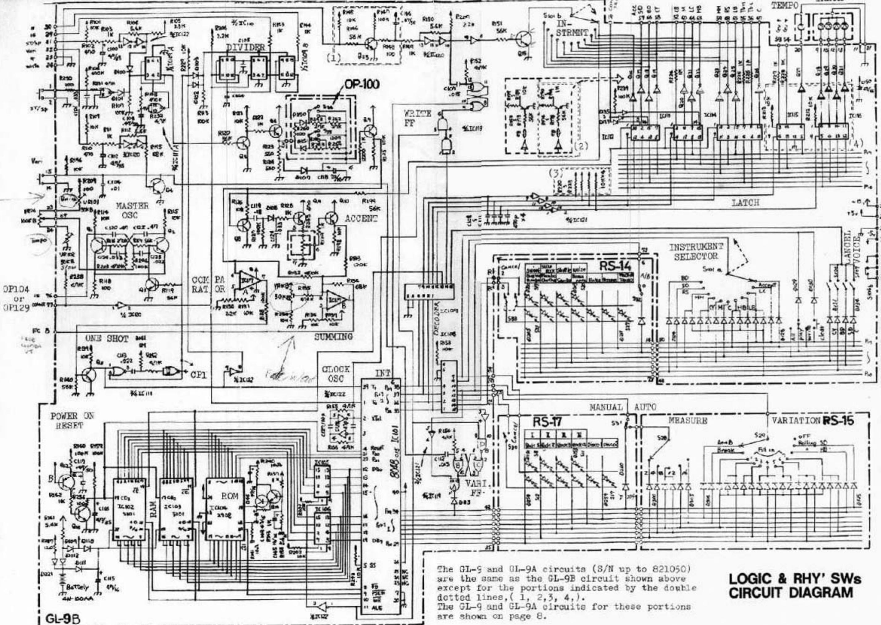
The GL-9 and GL-9A circuits (S/N up to 821050) are the same as the GL-9B circuit shown above except for the portions indicated by the double dotted lines, (1, 2, 3, 4). The GL-9 and GL-9A circuits for these portions are shown on page 8.
