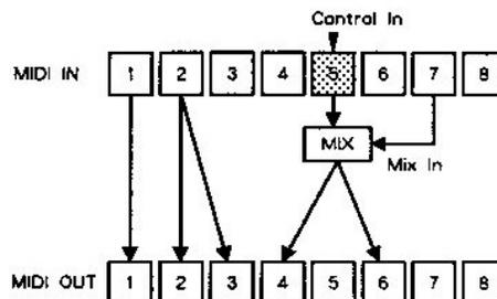
The Mix function does not allow you to input Real-time Messages to the two MIDI IN's at the same time.
