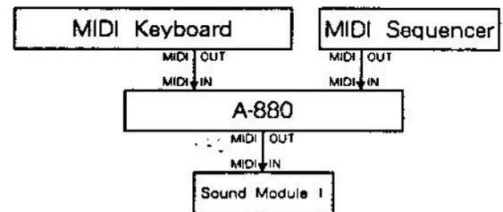
By using the Mixing function of the A-880, MIDI messages from the MIDI keyboard and sequencer are mixed and play the MIDI sound source.
