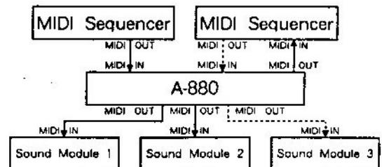
These two sequencers are used as a master and a slave. When they are synchronizing, the master sequencer plays the sound sources 1 and 2, and the slave sequencer plays the sound source 3.
