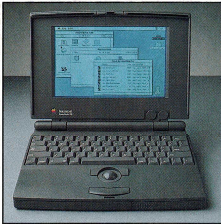
The Mac PowerBook 100, with built-in text processing, can write to ProDOS disks.
