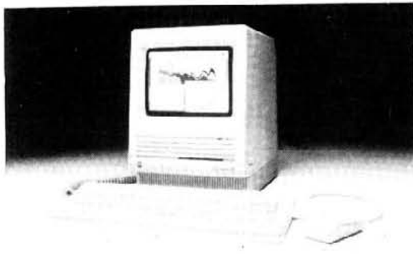
Macintosh SE with internal 20 Megabyte Hard Disk and single 800k Floppy Drive.
