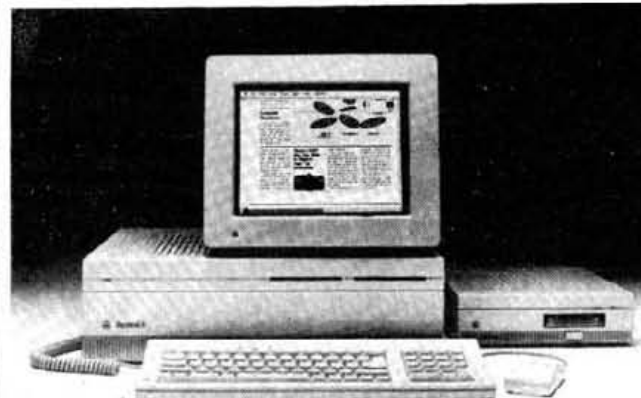
The new Macintosh II with internal 40 Megabyte Hard Disk and external Apple tape back-up.
