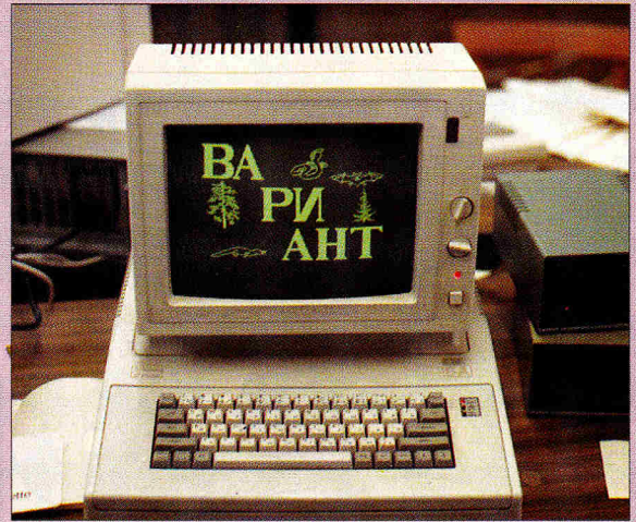
Variant's screen logo—Cyrillic version, of course. The Pravetz also supports the Roman alphabet.
