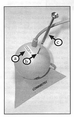
(c) or paper clip to push in on one of three plastic clips (d) (which will release easier with a little side force of the tool while depressing it), and thereby begin separating the case halves. The rest of the separating process was preformed by putting a large flat bladed screwdriver in the equatorial groove at various places and twisting the screwdriver, producing a muffled click. Unfortunately the plastic is soft and
