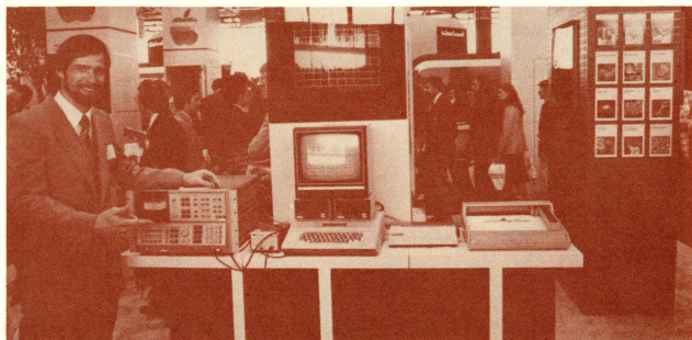
THE IEEE-488 INTERFACE CARD , a new product shown at NCC in Chicago, was demonstrated by Apple II Product Marketing Manager Mike Connor. The configuration used in the NCC demo - in which the card controlled a spectrum analyzer and a plotter - was also used to measure and analyze Apple II radio frequency emissions for the FCC.
