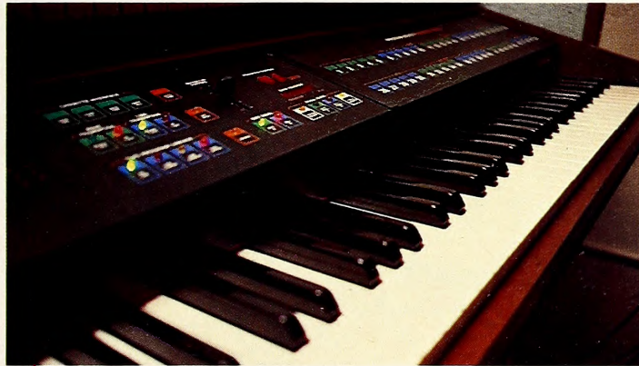
The Chroma music terminal from Fender/Rogers/Rhodes has a control panel with fifty presets and a keyboard that provides touch sensitivity.
