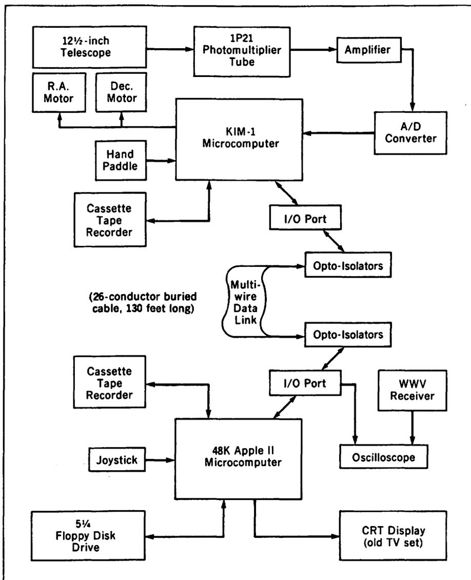
This flow chart summarizes the relationships between electronic and mechanical components. Everything in the upper half is located in the observatory, while the lower items are in the Skillman household. The analog-to-digital converter needs only 14 microseconds to change a signal level to its 12-bit representation. Each I/O port passes 10 bits in and 10 bits out. The WWV receiver is one of the Radio Shack TimeKubes.
