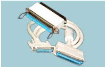
cable SCSI & terminators
