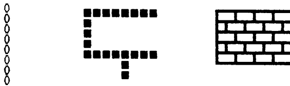
Figure 8–5 Pen pattern in memory and on the screen
