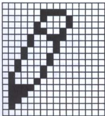
Figure 8-1. A screen image requires data in memory for each pixel, whether black or white.
